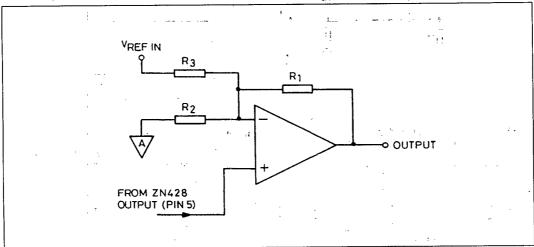
Fig.9 Bipolar operation - basic circuit
