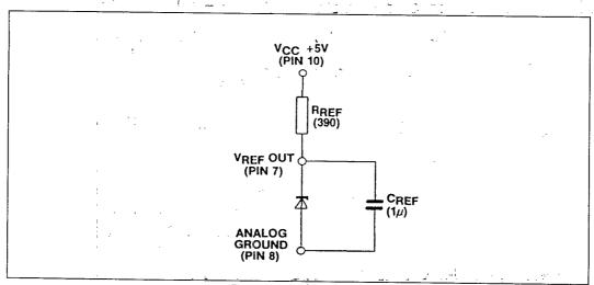
Fig.5 Internal voltage reference
