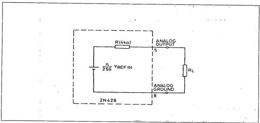
Fig.4 Analog output equivalent circuit
