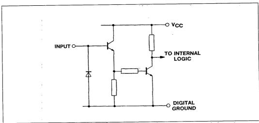
Fig.6 Equivalent circuit of all inputs
