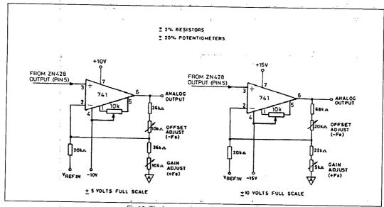
Fig.10 Bipolar operation - component values
