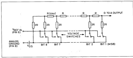
Fig.3 The R-2R ladder network
