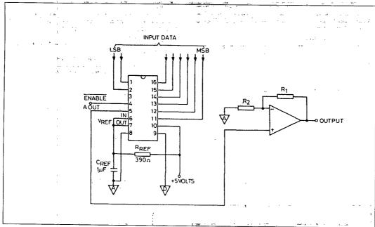
Fig.7 Unipolar operation - basic circuit
