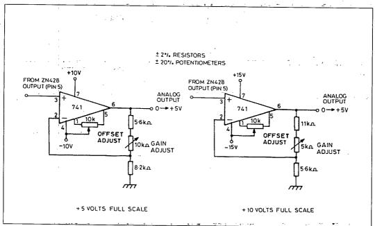
Fig.8 Unipolar operation - component values
